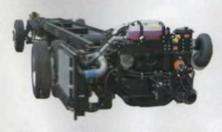
Freightliner Raised Rail 400 HP Cummins Diesel Pusher Chassis with side draft radiator and independent front suspension.
